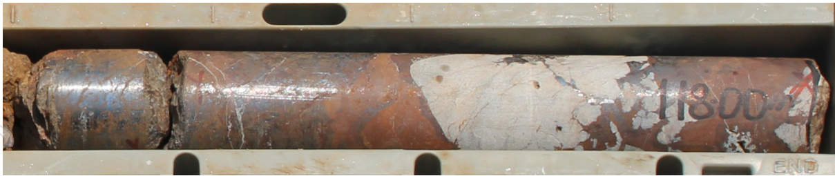
Photo 1 An example of very high-grade copper mineralisation 1 . Massive chalcocite (copper sulphide – steely, grey colour) and quartz (dull, light grey colour) with native copper (bronze colour). Dry, HQ (63.5mm diameter) core. NYDD053: 117.6m to 118.0m.
